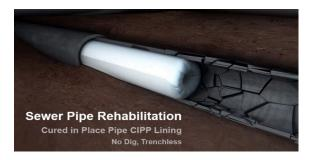
A cured-in-place pipe (CIPP) is a trenchless rehabilitation method used to repair existing Drains and sewers.
